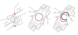
Remove the Panoramic Mount and attach the Magnetic Mount to the Pivo Pod.
