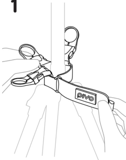
Wrap the strap around the center column of the tripod and pull the strap through the metal loop.
