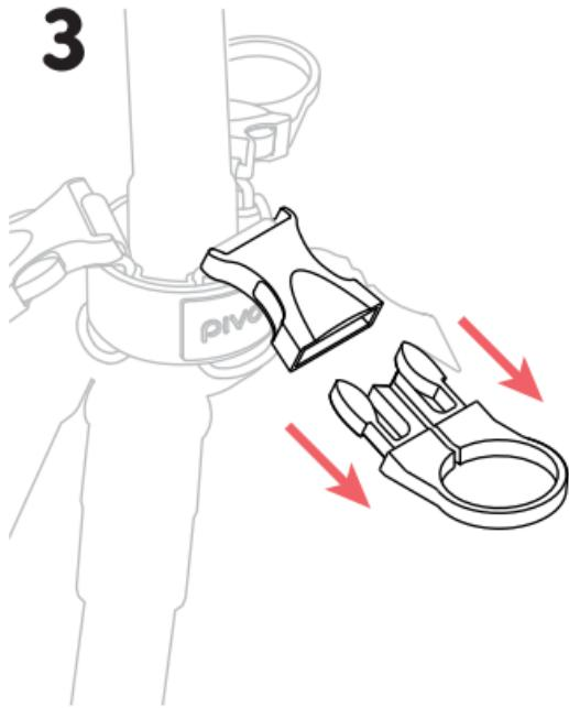
Unbuckle one of the clips and pull open the ring to fit over the water bottle neck.
